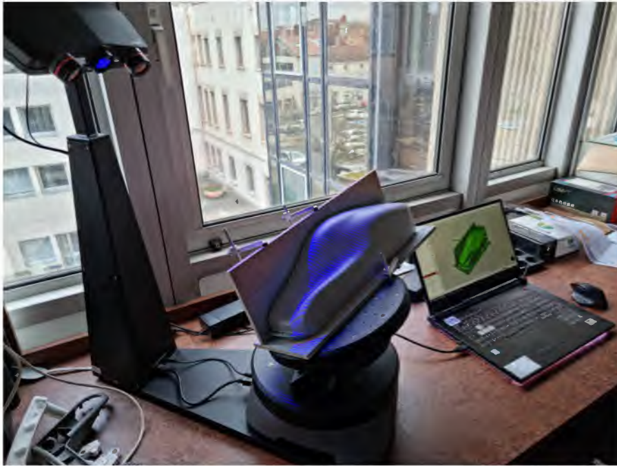
3D scan of a half maquette at FABLAB ROANNAIS AGGLOMÉRATION for digital imagery work and 3D printing of the full maquette at 1:8 scale for wind tunnel tests after full car body finish
