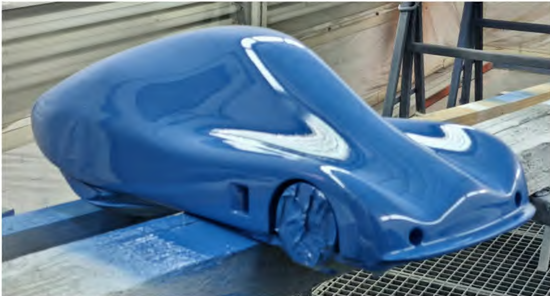
3D scan of a half maquette at FABLAB ROANNAIS AGGLOMÉRATION for digital imagery work and 3D printing of the full maquette at 1:8 scale for wind tunnel tests after full car body finish
